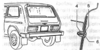
Fig. 18. Installation of Number Plates: 1, 6 — screws; 2, 5 — washers; 3 — nut; 4 — bushing
