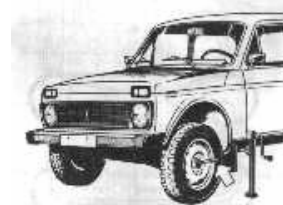
Fig 53. Jacking up car for replacement of wheels.
